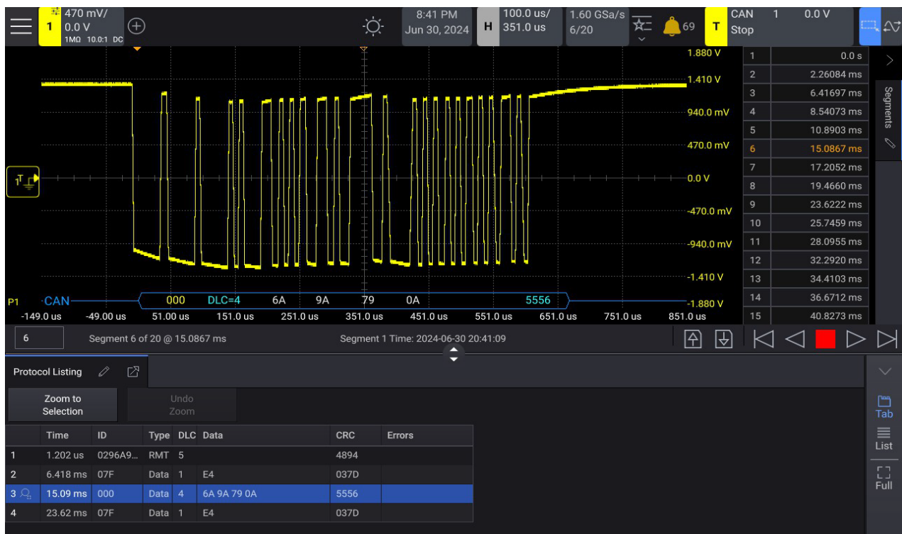
Figure 5. Segmented memory acquisition with automatic decoding selectively captures CAN packets with precise time-tagging between each occurrence
