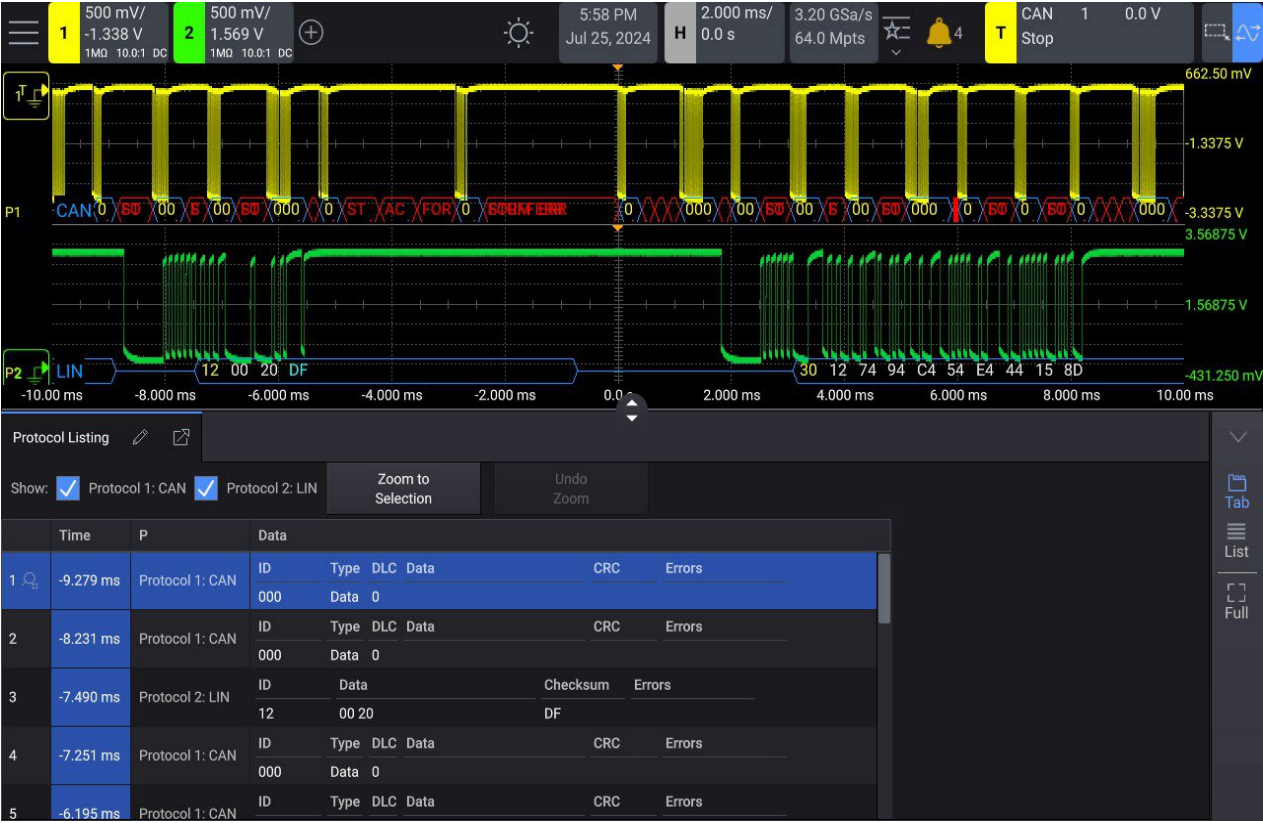
Figure 4. Dual-bus time-interleaved lister display makes it easier to track data through CAN-to-LIN gateways
