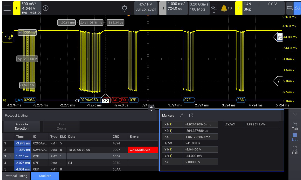
Figure 3. Hardware-based decoding captures and displays an infrequent CAN bit stuffing error followed by an error frame
