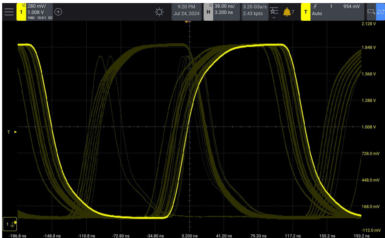
Figure 2. An update rate of 1.3 million waveforms per second easily captures infrequent glitches and jitter
