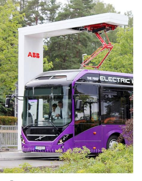
The OppCharge standard can be used for overhead charging, such as by Volvo electric buses. of today and the vehicles of tomorrow can leverage the same charging assets, regardless of power delivery capability or new feature sets within the vehicle, the charger, or beyond to the grid.
