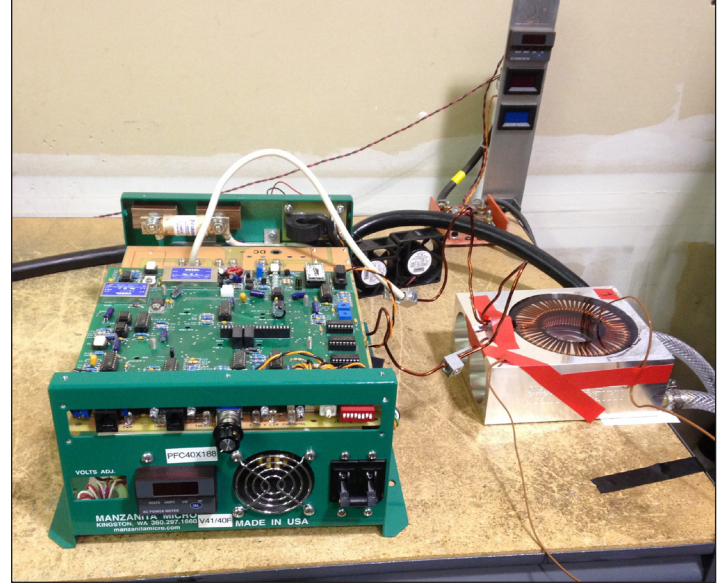
Figure 4: Test set-up for one SC-400 potted inductor showing the PFC40X-188 charger on the left, the potted inductor on the right, and the coolant inlet and outlet lines at the far right.
