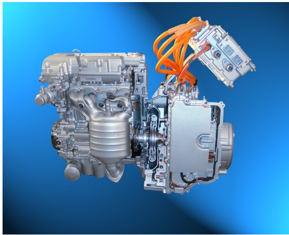
The Chevrolet Volt has a gasoline engine (left) as well as an electric motor/generator (right).
