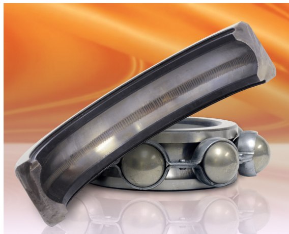
Fluted bearing race from a failed motor without shaft grounding protection
