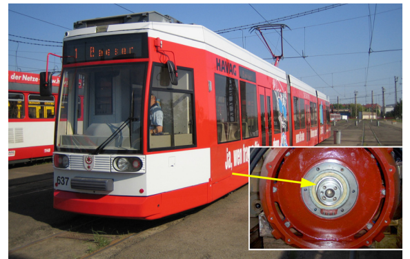
This all-electric tram in Halle (Saale), Germany, suffered bearing damage from inverter-induced voltages until the problem was solved in 2007 with the installation of an AEGIS™ SGR Bearing Protection Ring (inset) on the shaft of every traction motor in the fleet.
